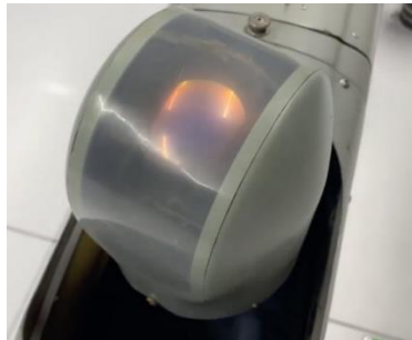
Left; Orlan 10 recovered in UKR in 2022, Right; close-up of TIR-only imaging pod on recovered Orlan 10
